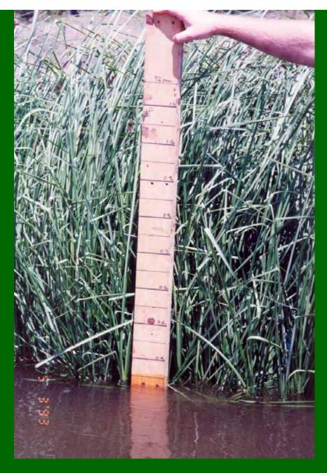
In a flume test a mature hedge can retain up to 40-45cm of water
